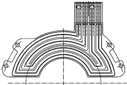
Figure 4: Cooling panel
