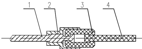
Figure 3: Clamping device. 1 – metal disk; 2 – metal clamp; 3 – graphite grips; 4 – converter element
