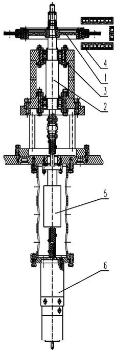
Figure 1: Sketch of prototype. 1 – rotating disk with converter; 2 – shaft; 3 – bearings; 4 – cooling panels; 5 – rotation feed-through; 6 – DC motor
