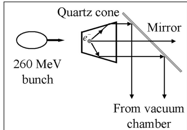
Figure 1: Scheme of quartz cone and mirror assembling.
