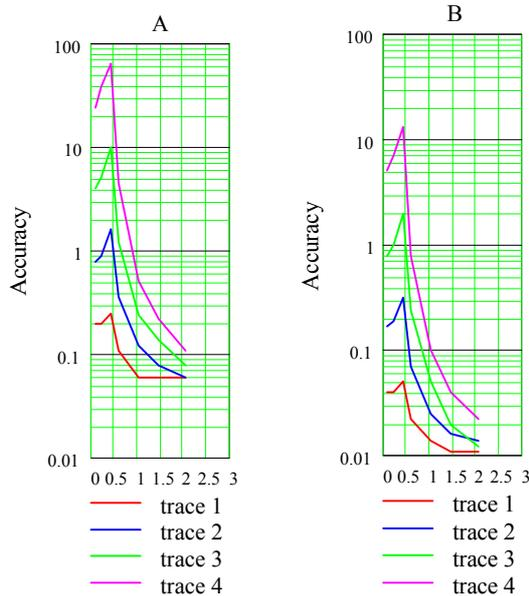
Fig. 3: Accuracy of the solution  $n(z)$  versus the parameter  $\alpha$  for different accuracy of  $\theta_y(x)$  measurement: A-0.05, B- 0.01. Different traces correspond to the different matrix sizes: 1-5x5, 2-7x7, 3-9x9, 4-11x11.
