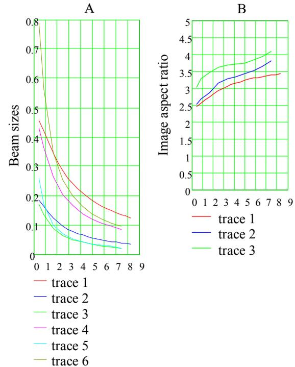
Fig. 4: Horizontal and vertical image sizes and image aspect ratio versus parameter  $\alpha$ .
