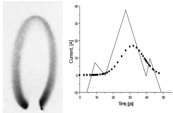
Fig. 2: Probe beam image on the screen and result of its processing. Solid curve represents the solution of linear system with  $7 \times 7$  matrix sizes (error is about 20%). Dots are a result of Gaussian curve fitting by special procedure.
