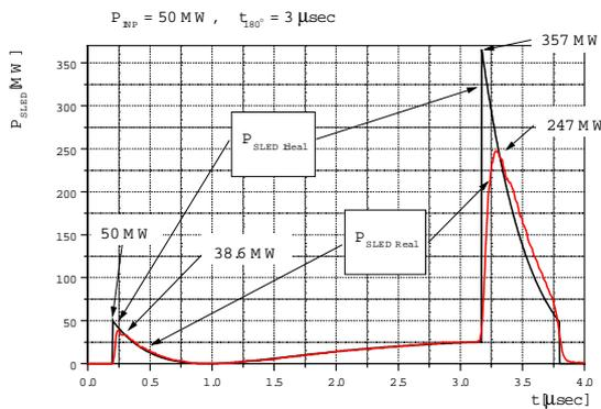
Fig. 4. Pulse shape after power compression system.
